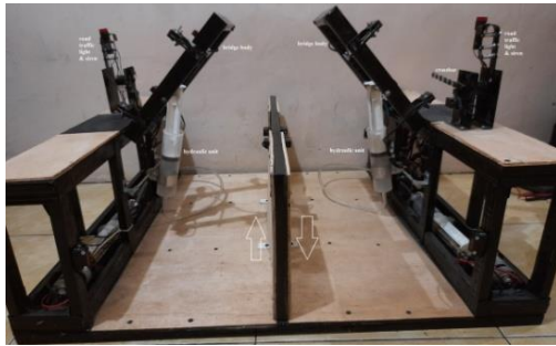
Figure 4. Installation of a Hydraulic System in the Development of a Miniature Bridge Frame
