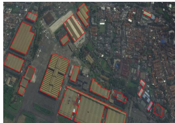
Fig. 4 Typical rooftops in Bandung City, with potential available rooftops for installation of solar panels are marked using red line
